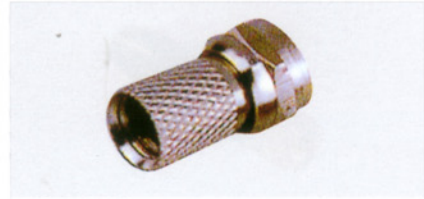
FC-A-0901 (0058R/6,0058R/7,0058R/58,0058R/59) 0058R/6:F plug for RG6 cable twist on type W/rubber ring 0058R/7:F plug for 5C2V cable twist on type W/rubber ring 0058R/58:F plug for RG58 cable twist on type W/rubber ring 0058R/59:F plug for RG59 cable twist on type W/rubber ring
