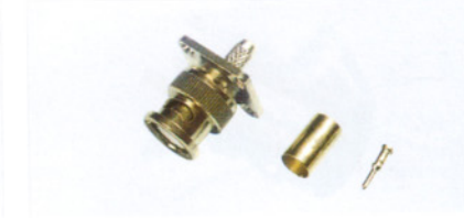
FC-A-0972 (0204/58,0204/59) 0204/58:BNC plug for RG58 cable chassis mount crimping type 0204/59:BNC plug for RG59 cable chassis mount crimping type
