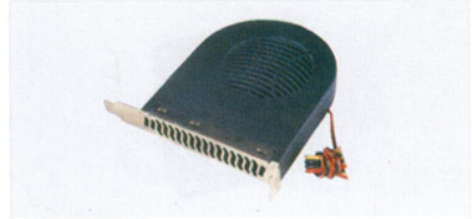
FC-B-0018 (SB-A) System EXhaust Blower Hot air is drawn into the fan and expelled through the metal vent, out of the case Voltage: DC 12V Noise: 23dB Current: 0.15A Speed: 3000RPM±10%
