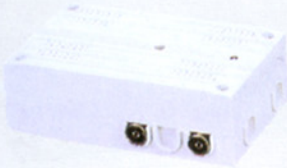
FC-B-0536 (TY313) Band width:40-860MHz Max GAIN:27dB OUTPUT:2way 75Ω(9.5mm TV socket)
