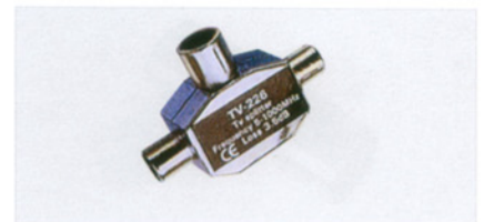
FC-A-0886 (5072) 2way splitter 5-900 MHz 9.5mm jack to 2x9.5mm plug die-cast
