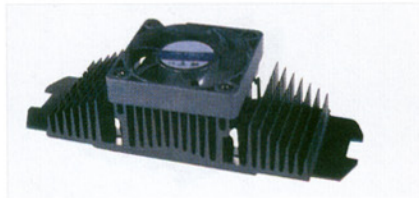
FC-B-0019 (PIII-300C) For CPU: Intel PIII/PIII to 700MHz DC 5010 FAN Voltage: DC 12V Noise: 26dB Current: 0.12A Speed: 6000RPM±10% Sink: 47x137x25mm Supporting Detection Of The Rotating Speed Of Fan
