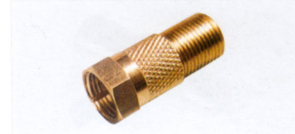
FC-A-0937 (0073A,0073A/MU,0073A/UM) 0073A:F plug to jack adaptor 0073A/MU:M10x0.75mm F plug to 3/8-32 jack adaptor 0073A/UM:3/8-32 F plug to M10x0.75mm jack adaptor
